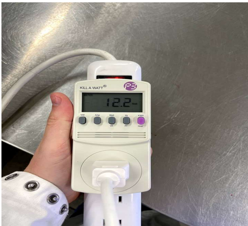
Image 2: Kill-A-WATT reading when device is on.
